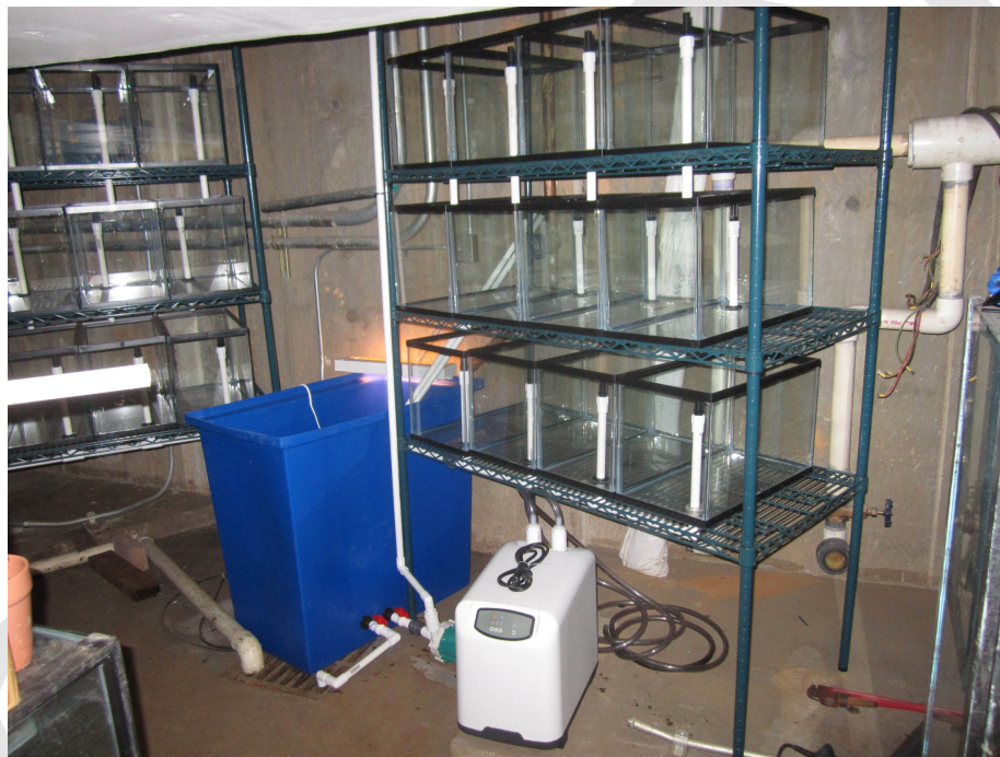
Figure 3. This is the laboratory housing for the set of Dougherty Plain Cave Crayfish that bred in captivity (without water in the system here). Note the three shelves, each with 4 37.85L aquaria. The top two shelves spill into the tanks below them through standpipes and bulkhead fittings. The bottom shelf drains through PVC pipe to the central filtration unit (blue tub). The white unit is the TECO® brand TC20 inline water chiller, maintaining the system at a constant 20°C. Photo by Danté D. Fenolio.
